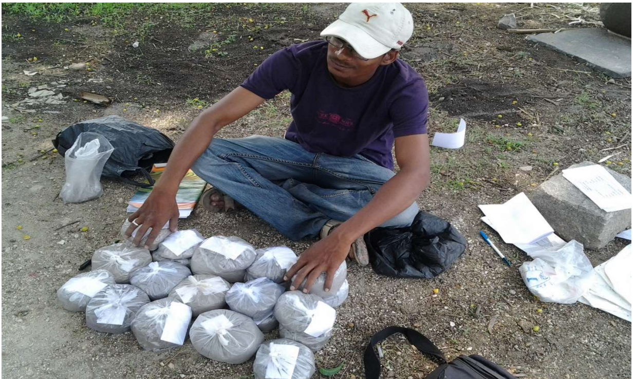
Soil samples for testing bagged and labeled
